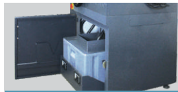
Recirculating Coolant Tank
