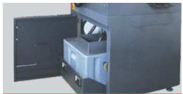
Recirculating Coolant Tank
